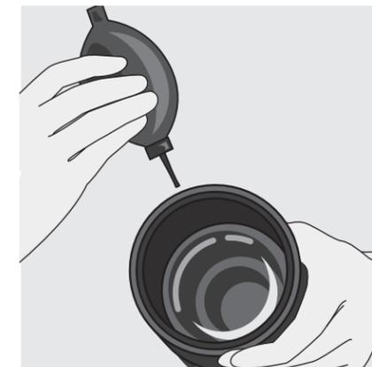
First, remove the lens cover and brush the dust from the lens surface with a soft brush or blower brush.
