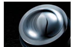
Metal mold for producing the aspherical lens
