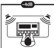
If the monitors are close to the back wall, try setting the Acoustic Space switch to -2 dB for less attenuation.
