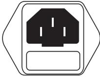
**IEC Power Connection:** Your Eris E5/E8 accepts a standard IEC power cord.
