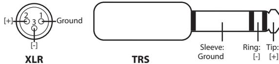
**Power User Tip:** If your audio source provides balanced XLR or ¼" TRS (tip-ring-sleeve) outputs, use one of the corresponding balanced Eris inputs, since balanced cables are resistant to induced noise from radio-frequency or electromagnetic interference (RFI or EMI). If the audio source has unbalanced ¼" TS (tip-sleeve) outputs, use a ¼"-to-RCA adapter or adapter cable. Always use the shortest cable possible to minimize the risk of induced RFI or EMI noise.
