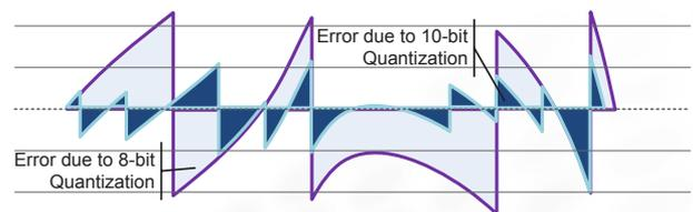
**Figure 2 – Comparison of quantization errors.**
