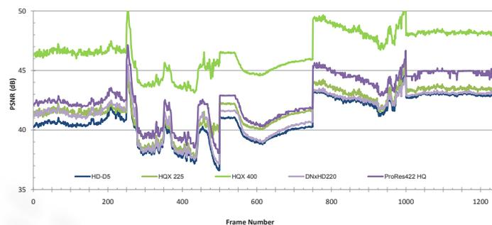
**Figure 7** – PSNR comparison of 5:1 class codecs, and HQX at 3:1.
