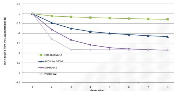
**Figure 9** – Multi-generation performance of intermediate codecs.
