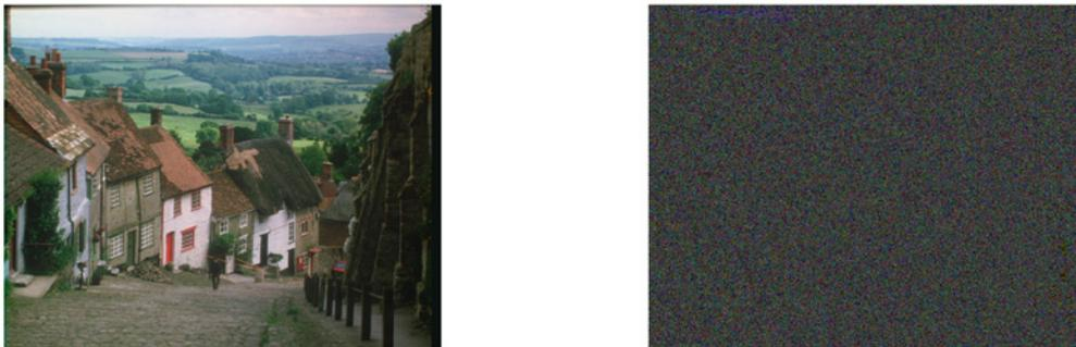
**Figure 4** – A picture and the noise in its bottom two bits.
